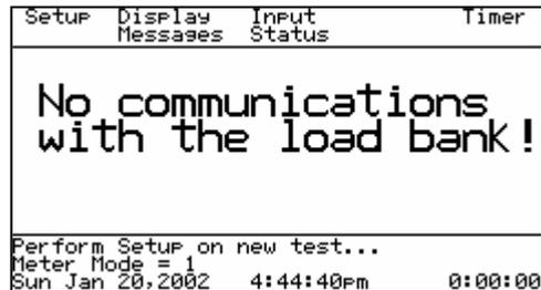
Once power is present, and the "Enter" key is pressed to clear the splash screen on the *Local Control Panel*, a screen similar to the one shown will be displayed.
